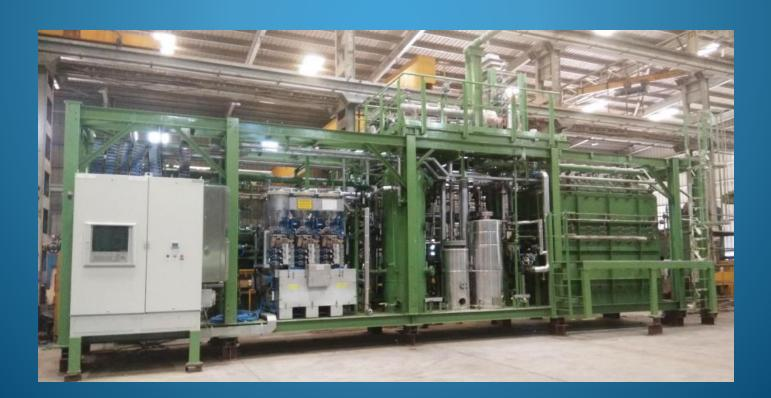
Packaged Hydrogen Plants 2 No. Hydroprime HC-300 for Samsung Korea 330 Nm3/Hr
